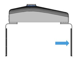
Consider the presence of the force sensor when the workpiece is aligned by using the fingers of the gripper or when the workpiece is picked sideways since the gravity can affect the force measurement.
