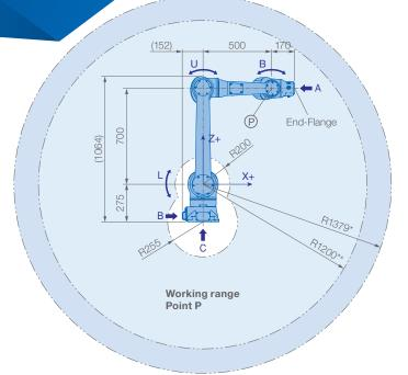
Absolute reach: S/L-Axis center of rotation to R/T-Axis center of rotation Effective reach: S/L-Axis center of rotation to Point P \*\*
